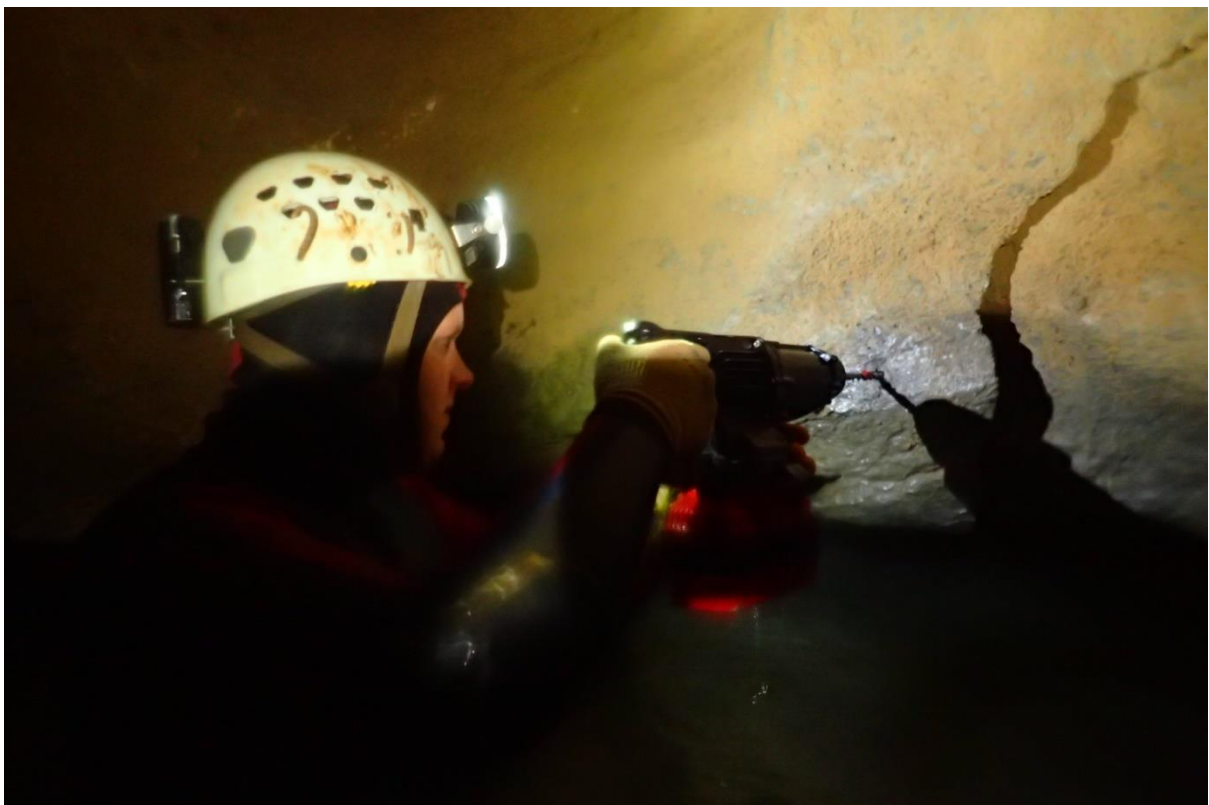
2. Using submersible drill
